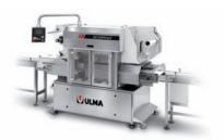
Scorpius 600 with a Sercom tray denester showing a Cryovac Mirabella® application for fresh meat. Cryovac Mirabella® is a patented packaging concept which allows product-to-film contact without discolouration. Instead of wasted headspace, the product can reach the level of the tray flange.
