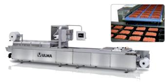
New range thermoformer TFS 700 integrated with VEMAG portioning machine for minced meat. The new efficient monitoring software will show the data captured from the installation.
