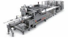
A FLOW-VAC®, the vacuum packaging system that adapts to the length of each product in an automatic line. The application is based on our FV 35 integrated with an indexing feeder (Sealed Air) and a rotary vacuum chamber VR8620-14 (Sealed Air). A suitable vacuum packaging solution for smoked and processed meat and also cheese.
