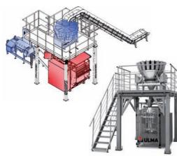
The VTC 700 high performance continuous VFFS machine, integrated with a product lifting conveyor and a Scanvaegt (Marel) multihead weigher for frozen nuggets packaging. Installation is completed with checkweighing
